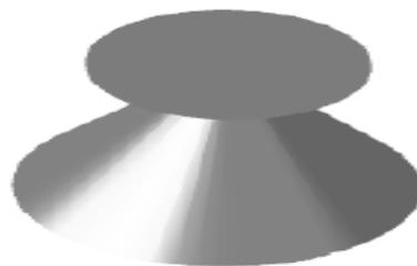
**Figure I.9:** Antenne discône [I.11].
