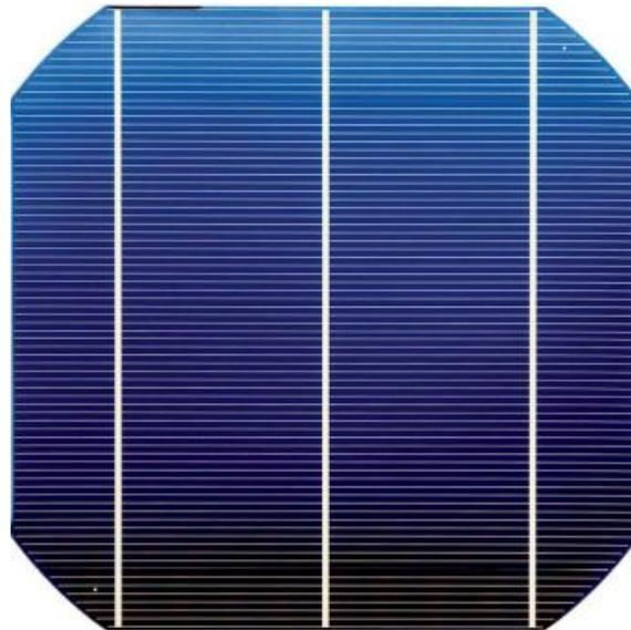
*Figure 2.5 : Cellules monocristallines [39]*
