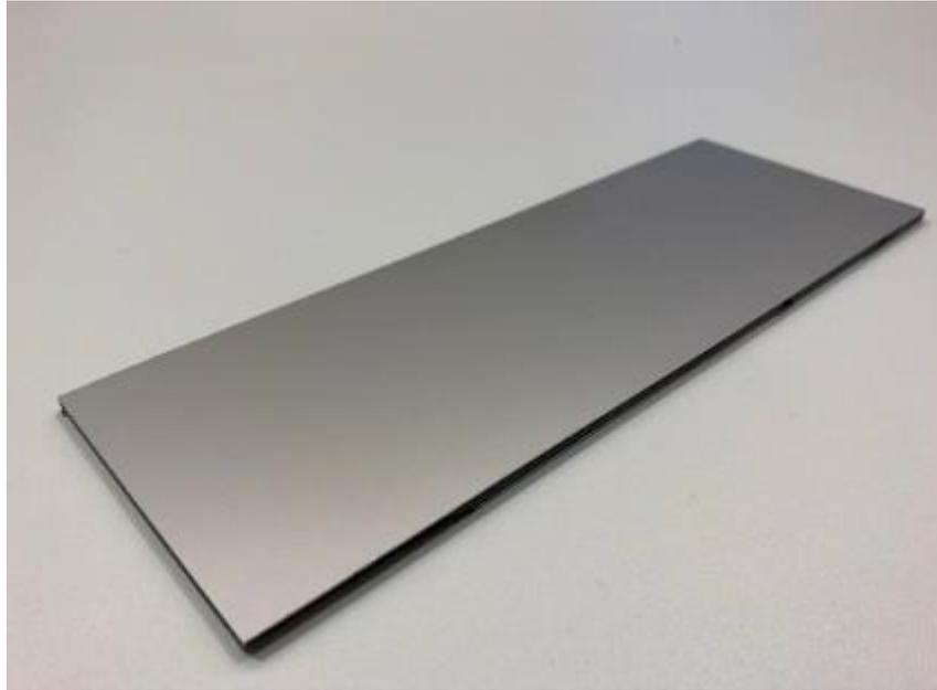
*Figure 3.7 : Alucobond (<https://www.aikolon.fi/en/products/composite-materials/alucobond-pe>)*
