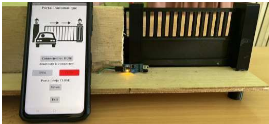
Figure II. 53:Portail déjà CLOSE.
