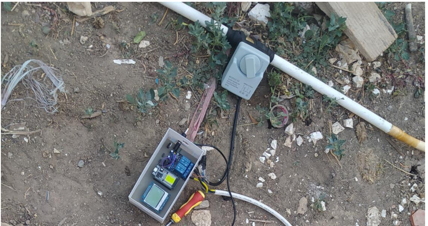
Figure III-23: Demonstration of the solenoid valve in function seamlessly connected to the board.
