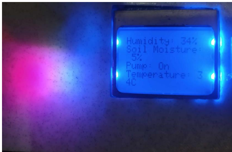
Figure III-26 : Nokia 5110 Displaying Sensor values
