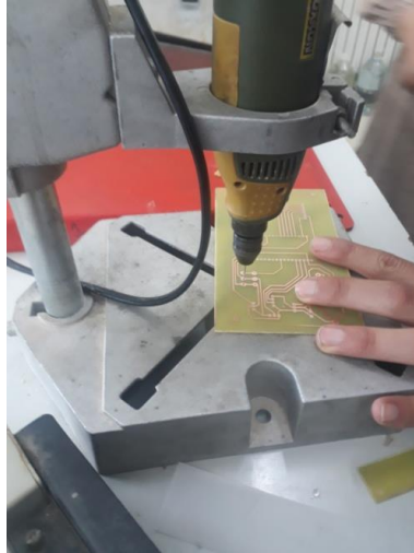
Figure III-6: Drilling the PCB
