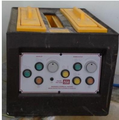
Figure III-5 : PCB chemical etching
