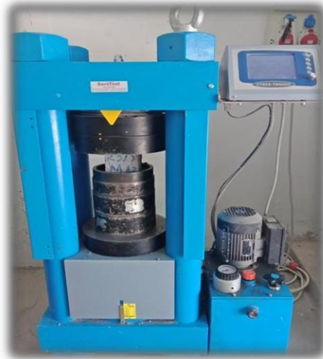
*Figure III.15 Essai compression*
