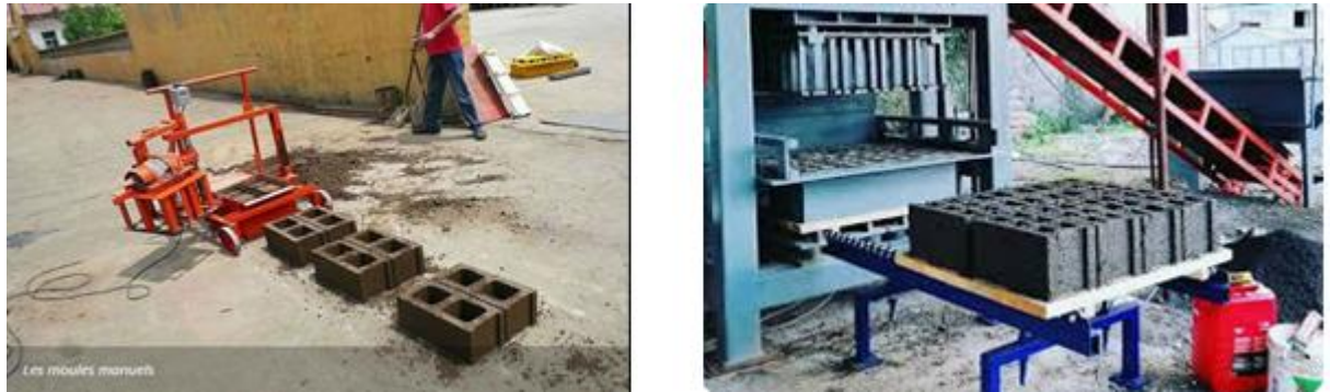
Figure II 2: Fabrication des hourdis
