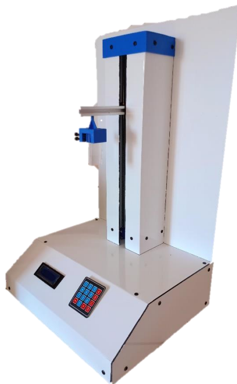
Figure III.14 : prototype de machin dip coating real
