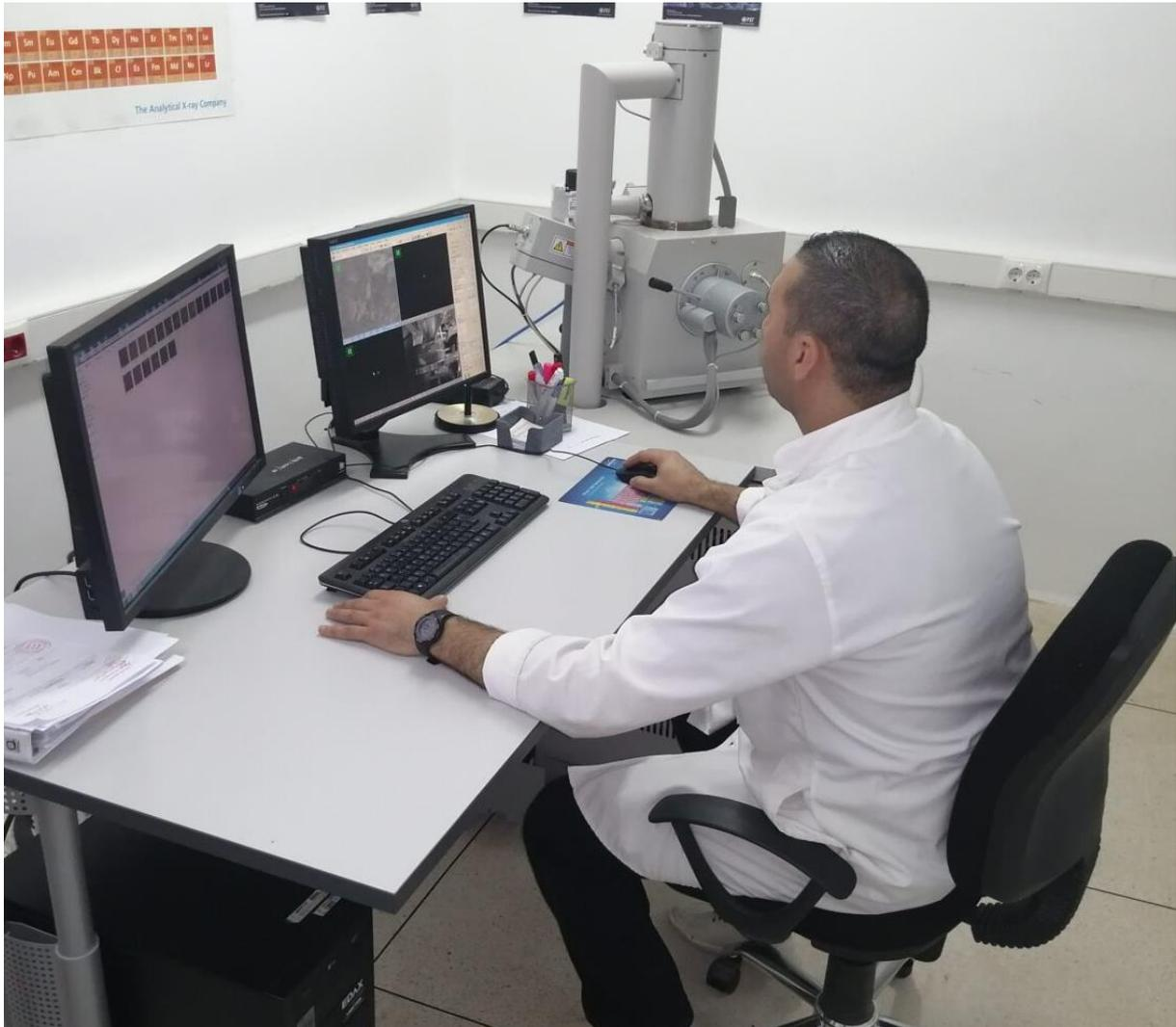
**Figure a.06: Scanning Electron Microscope (SEM) Inspect S-50.**
