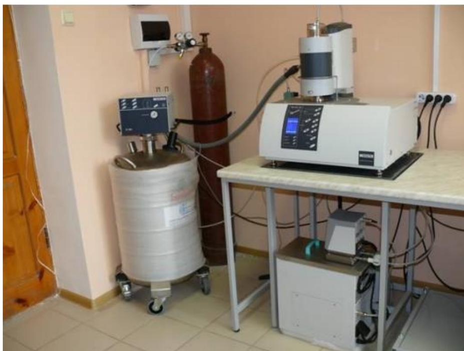
**Figure a.05:** Simultaneous Thermal Analyzer –STA 449 F3 Jupiter.
