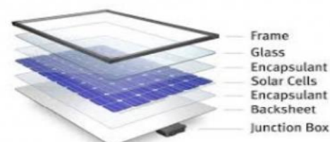
Figure 6: Structure of solar panel
