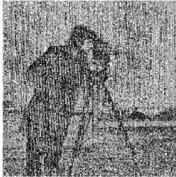
Figure 2.25 : Result of Received Picture with 3-taps and SNR = 20 dB
