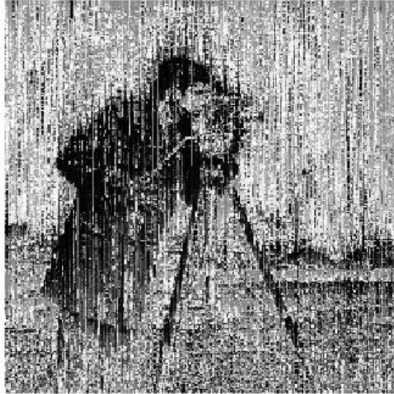
Figure 2.21 : Result of Received Picture with 3-taps and SNR = 35 dB
