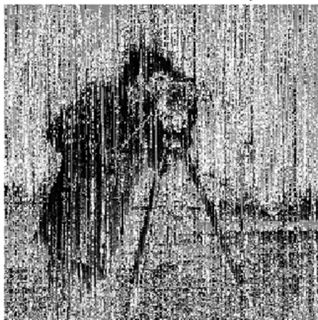
Figure 2.24 : Result of Received Picture with 3-taps and SNR = 20 dB
