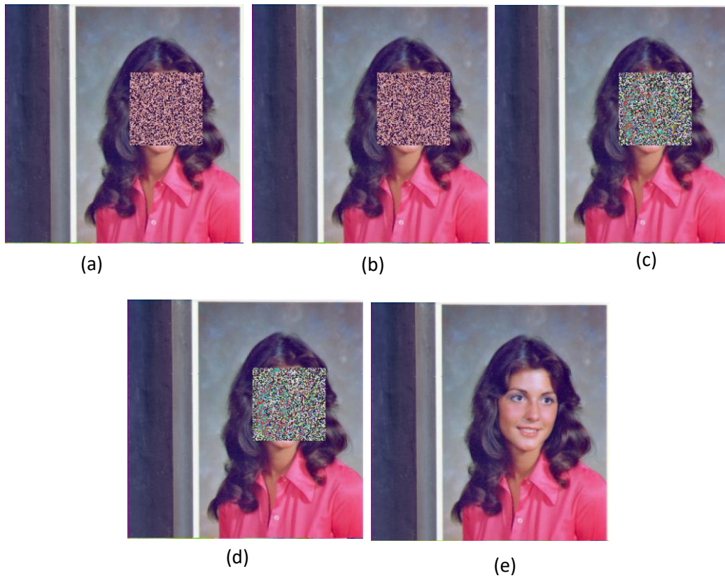
Figure .27. Sensitivity test: Decrypted face of image 4.1.04.tiff for (a) x'_0 = x_0 + 10^{-16} (b) r'_0 = r_0 + 10^{-15} (c) x'_1 = x_1 + 10^{-16} (d) r'_1 = r_1 + 10^{-15} (e) With correct key.
