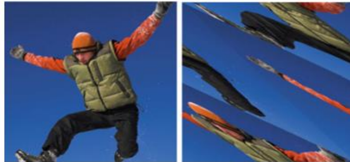
Figure. 11. example of confusing using Arnold Map a original image b 1st Iteration.
