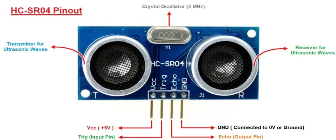
Figure II. 3: ultrasonic HC-SR04 sensor pinout.
