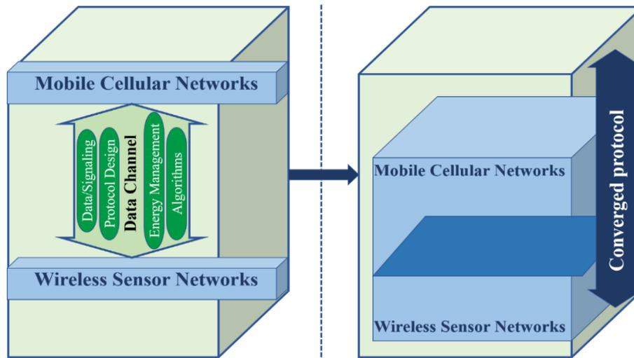
Figure 3.11 Protocol stack for WSN and MCN convergence network.
