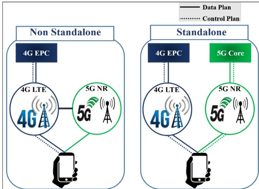
Figure 3.2 Non-Standalone and standalone deployment.
