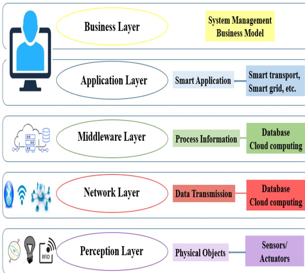
Figure 2.3 Five-Layer IoT Architecture.
