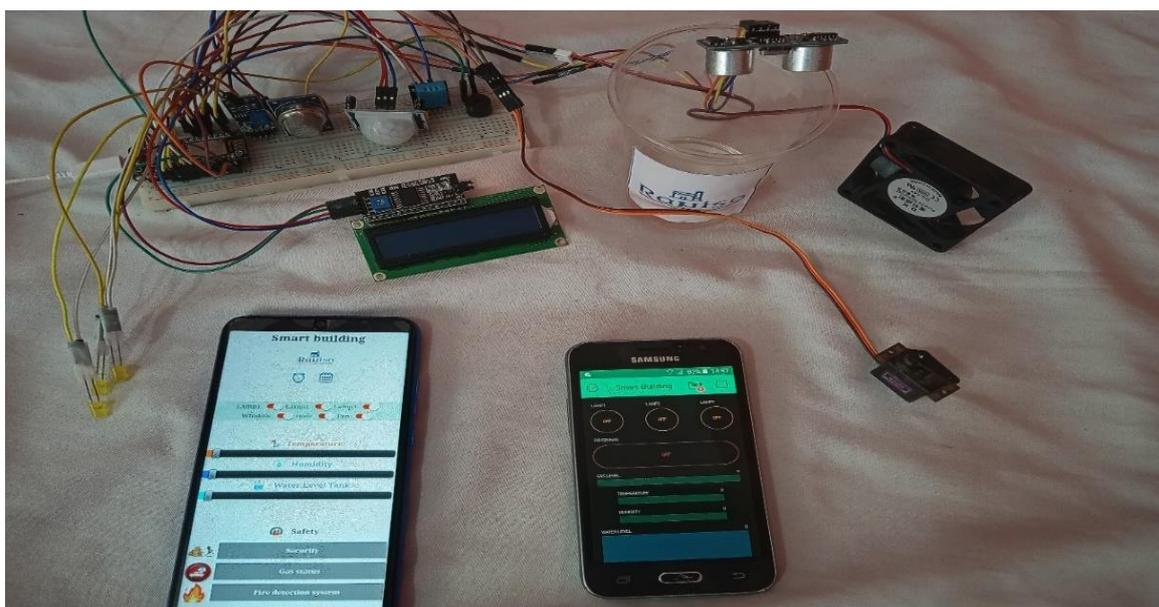
Figure 4.14 A practical proposal for the smart environment system based on two IoT/M2M platforms.
