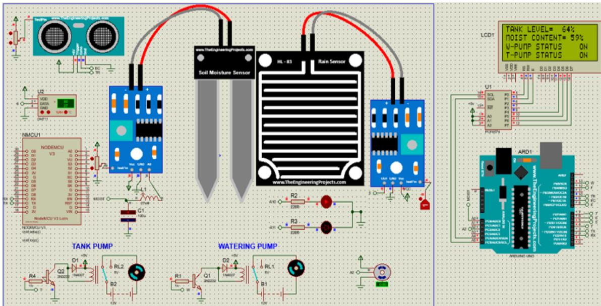
Figure 4.24 Schematic of the smart farming system simulated with Proteus.
