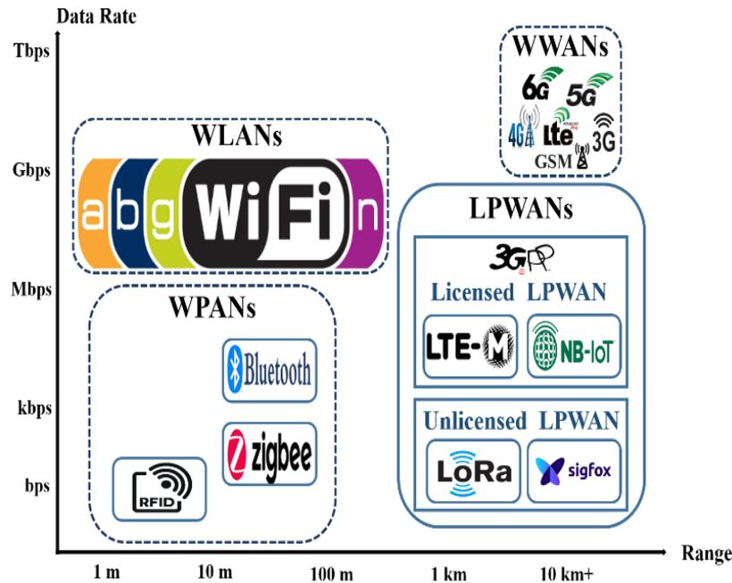
Figure 2.7 IoT/M2M communication technologies.
