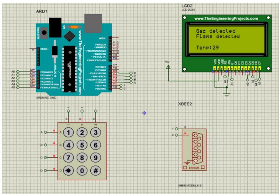
Figure 4.5 Virtual installation of the remote control system.
