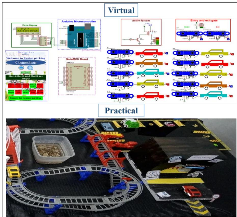
Figure 5.4 The proposed system prototype for smart parking.
