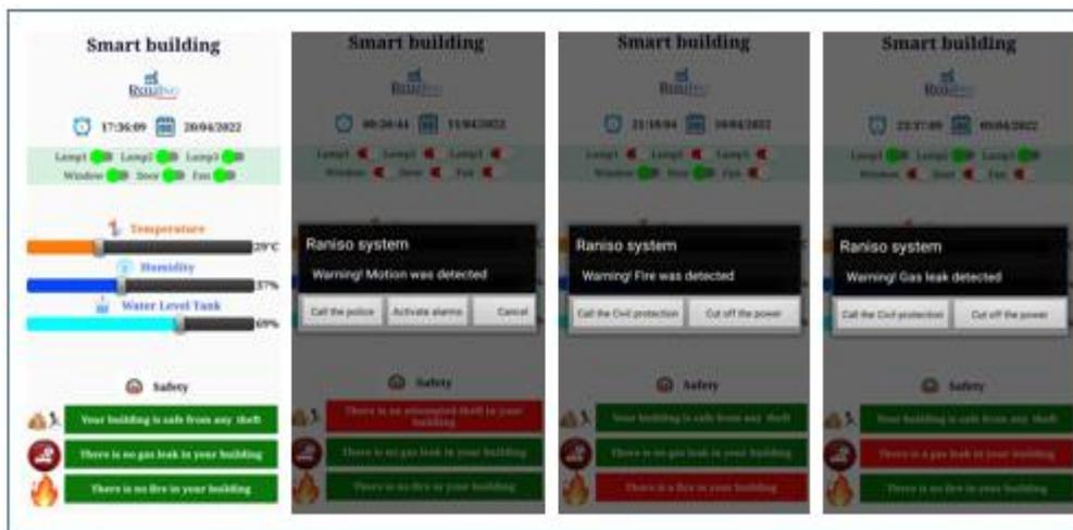
Figure 4.15 The user interface of the Raniso App in different conditions.
