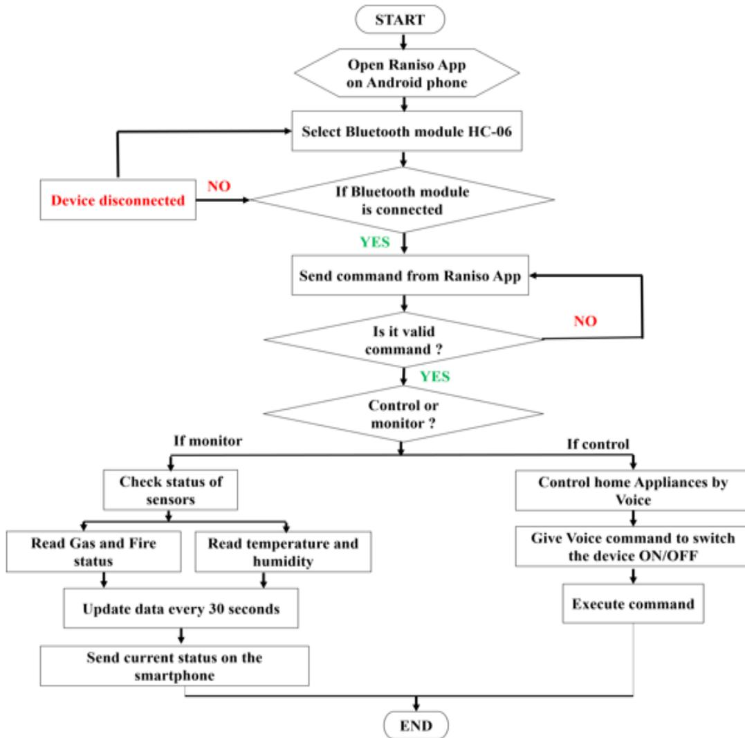
Figure 4. 7 Operational flowchart of the smart home automation system.
