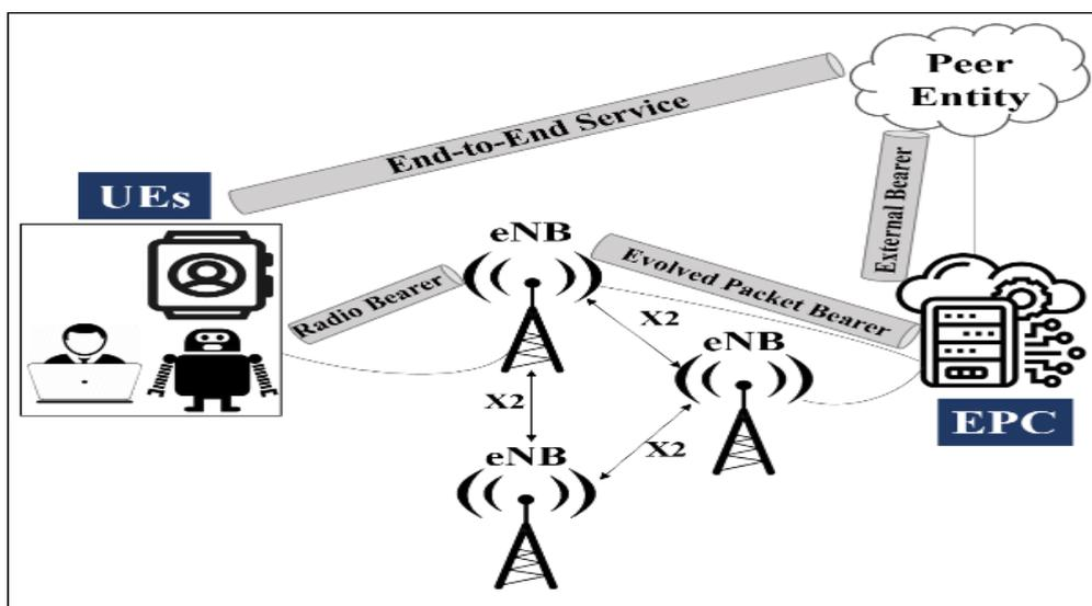
Figure 2.10 End-to-End QoS scheme in 4G LTE network.
