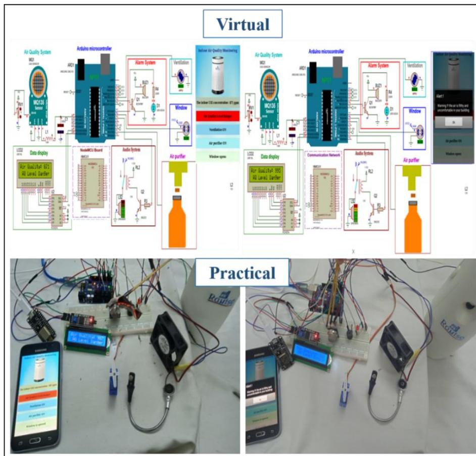
Figure 5.27 Indoor air quality monitoring system.
