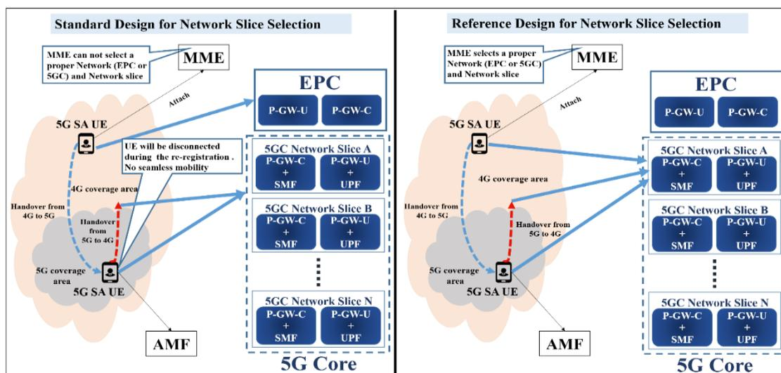
Figure 3.7 Standard and Reference Designs for Network Slice Selection.
