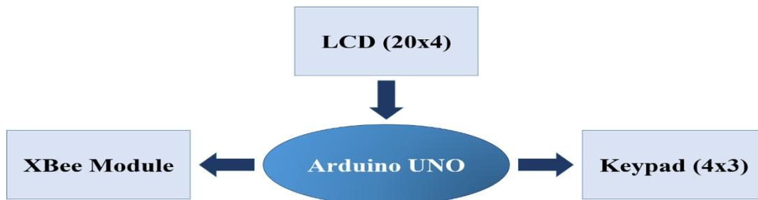
Figure 4.2 The block diagram of the remote control system.
