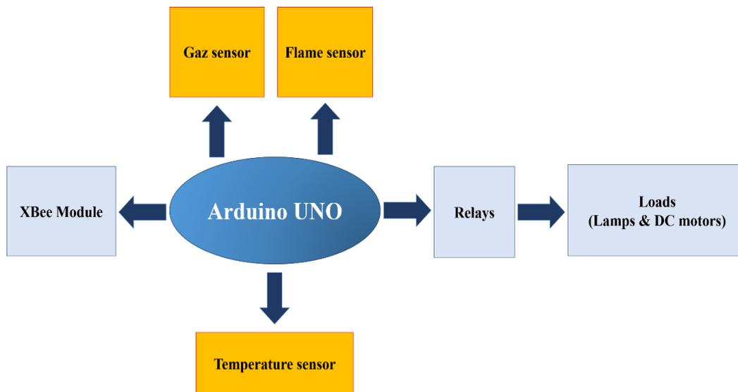
Figure 4.3 The block diagram of the master control board system.
