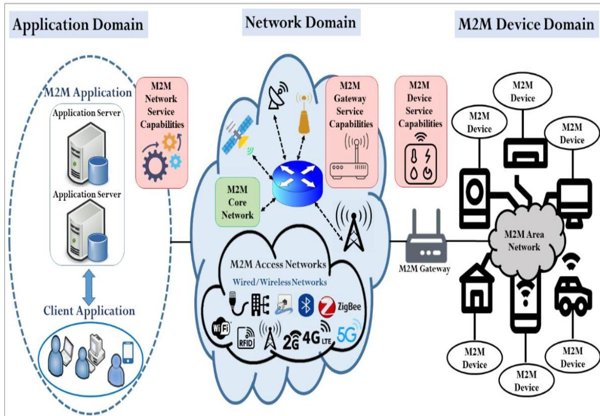
Figure 2.5 The architecture of M2M communication.
