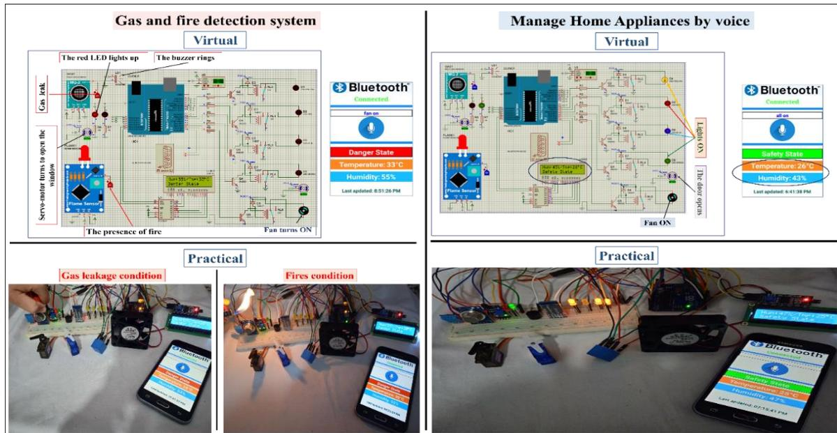
Figure 4.11 Implementation of M2M smart home automation.
