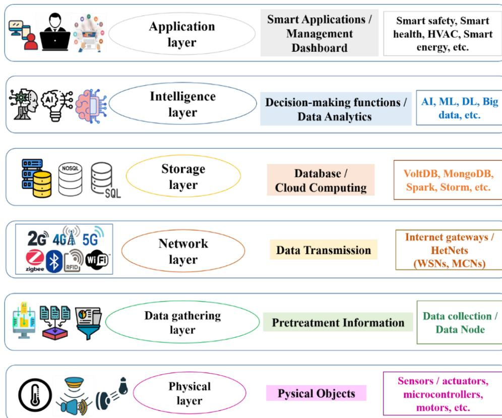
Figure 5.2 AI based IoT/M2M smart building layer system architecture.
