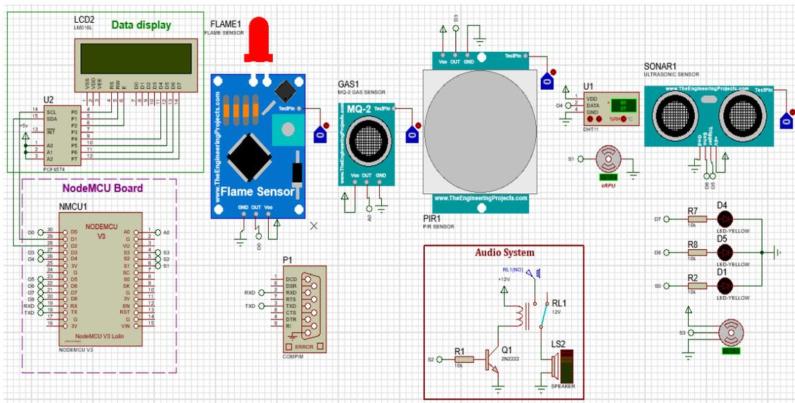
Figure 4.13 Circuit diagram of the smart environment system simulated using Proteus.
