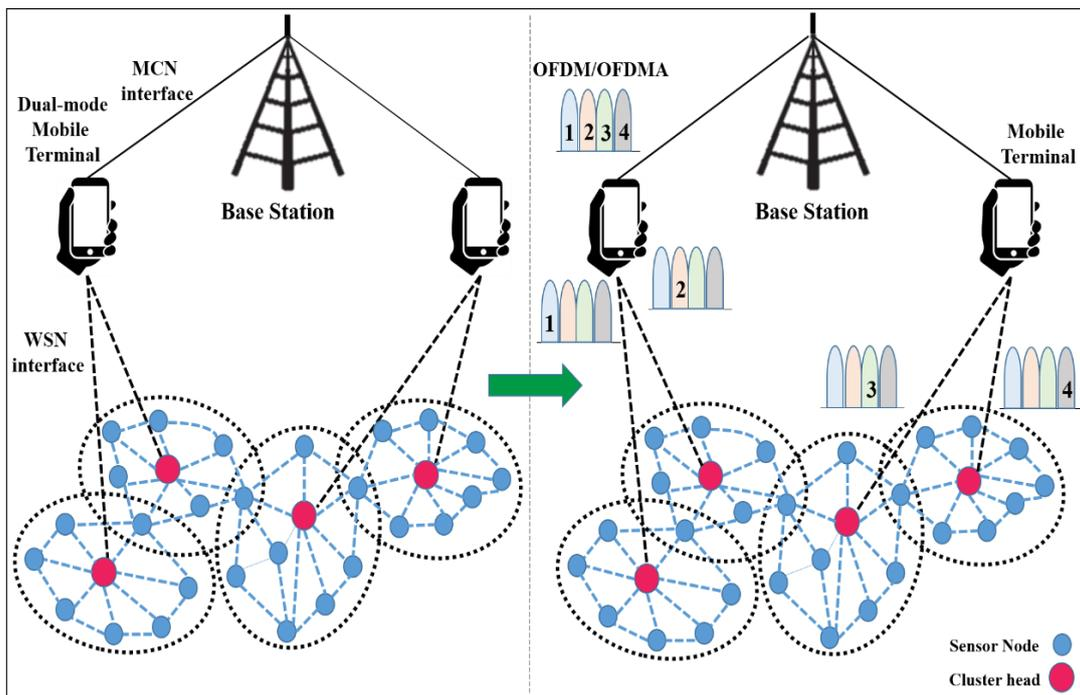
Figure 3.10 Converged air interface for WSNs and MCNs.
