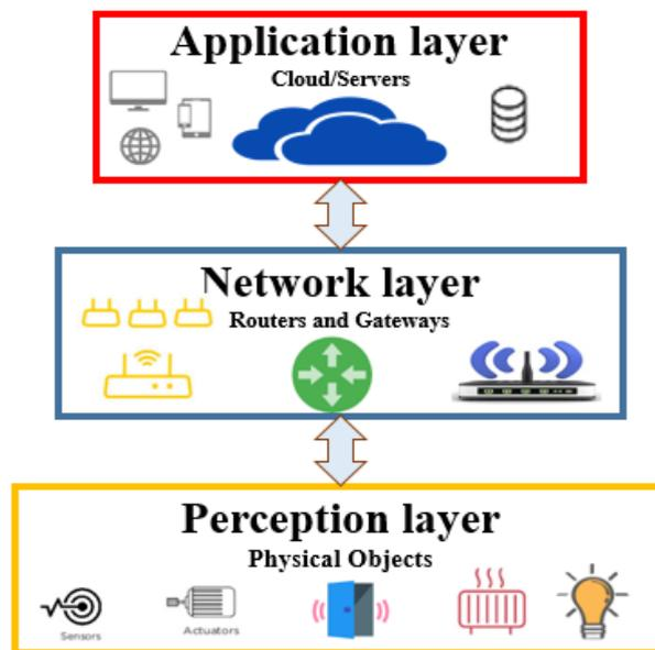
Figure 2.2 Three-Layer IoT Architecture.
