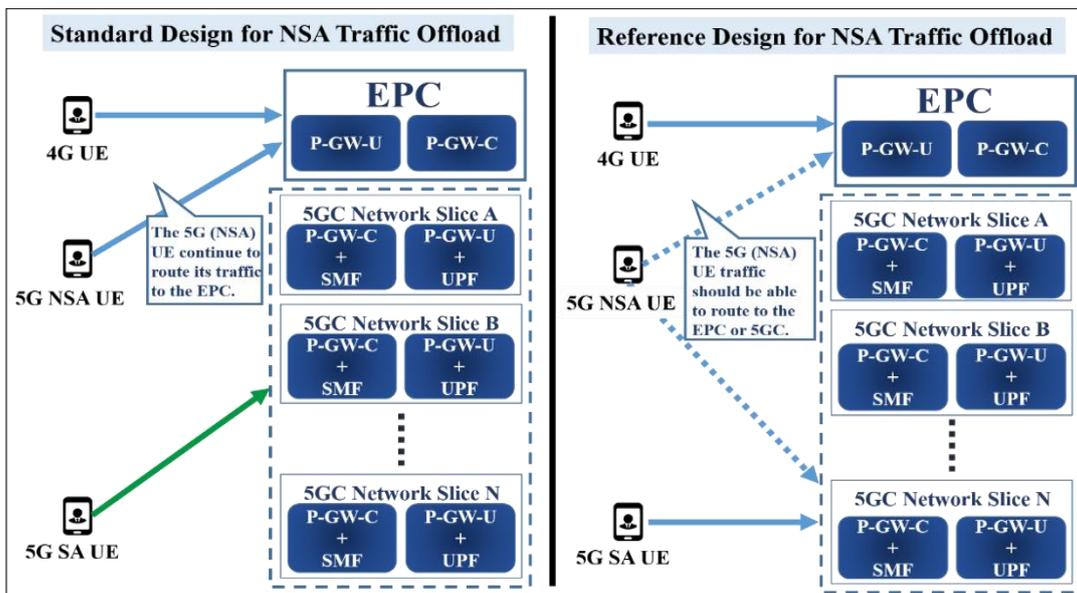
Figure 3.8 5G NSA UE Traffic Offloading.
