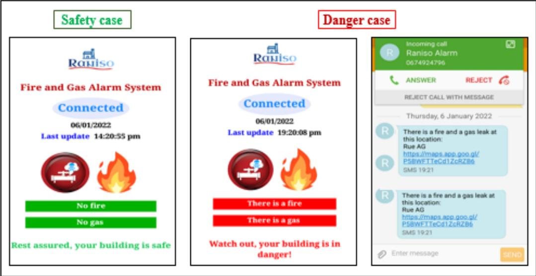
Figure 5.19 Fire and gas detection interface on the Raniso App.
