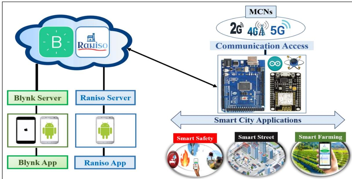
Figure 4.18 System design architecture.
