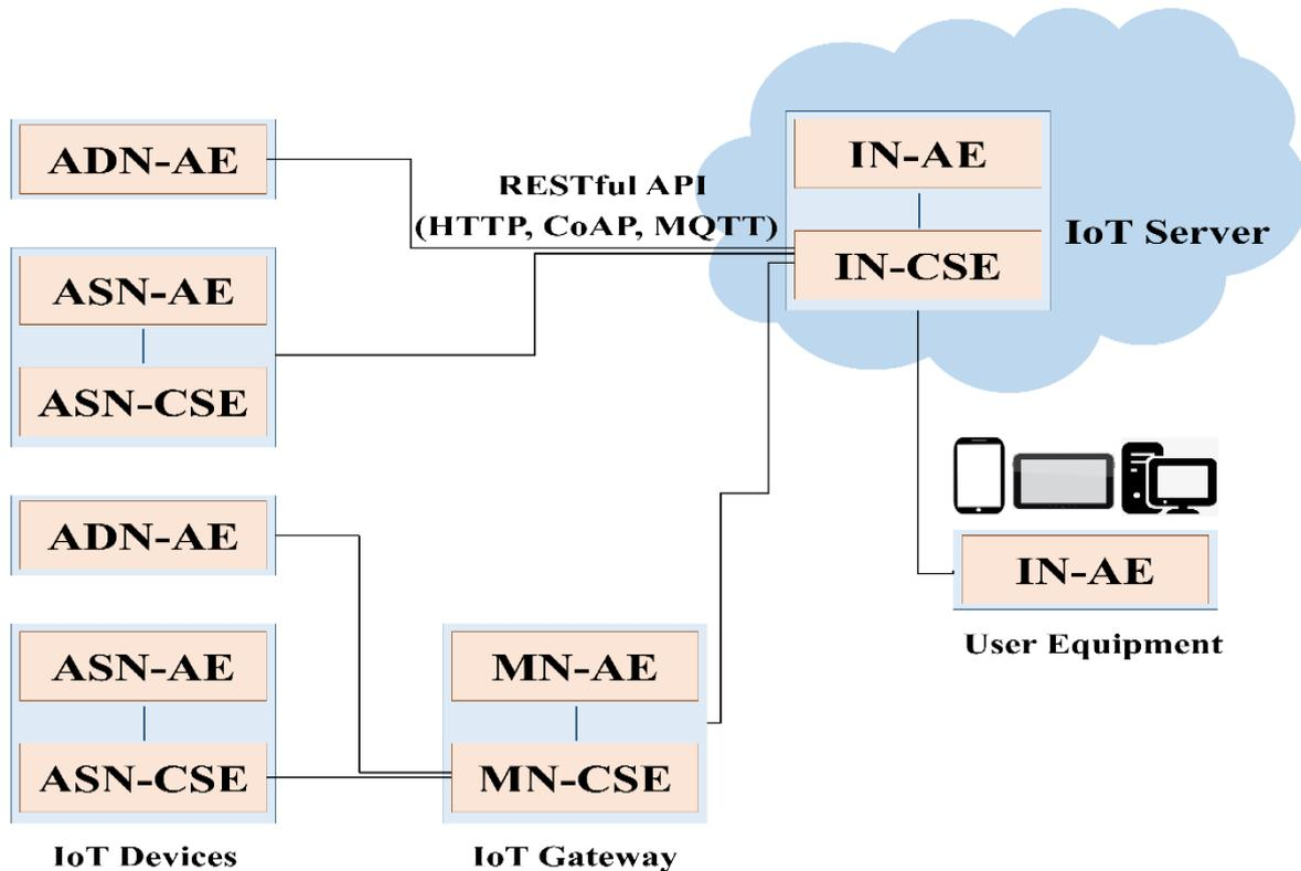
Figure 2. 6 OneM2M reference architecture model.
