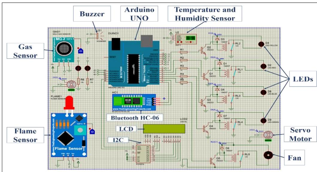
Figure 4.10 Scheme of M2M-Smart home automation.
