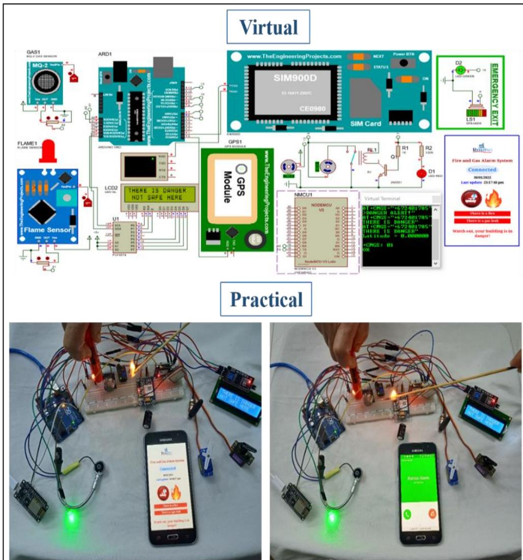
Figure 5.18 Fire and gas alarm system.
