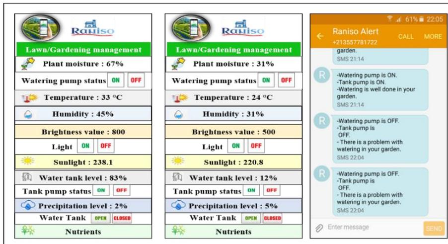
Figure 5.8 Garden irrigation automation interface on the Raniso App.
