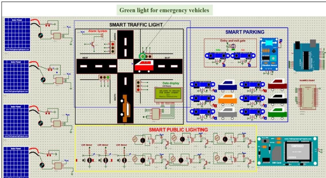
Figure 4.22 Schematic of the smart street system simulated using Proteus.
