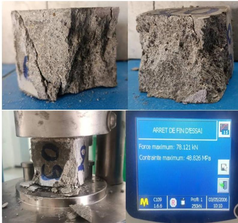
Figure 29: essai a la compression
