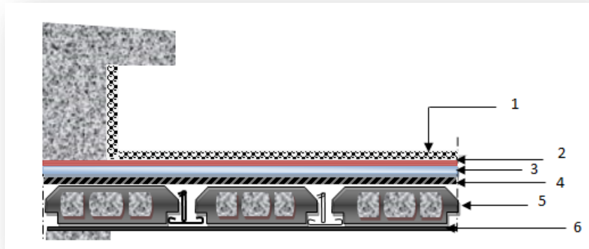
Figure II.9. Plancher terrasse inaccessible
