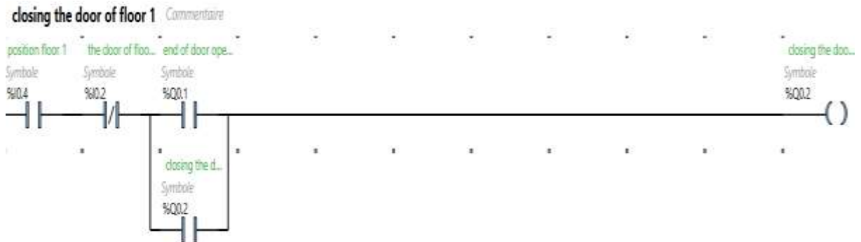
Figure III.8. 1st floor door closing
