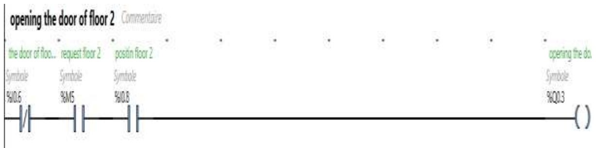
Figure III.11. 2nd floor door opening
