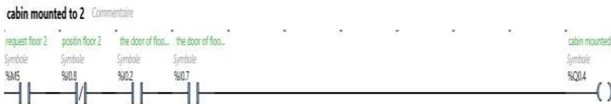
Figure III.7. the cabin amount to floor 2
