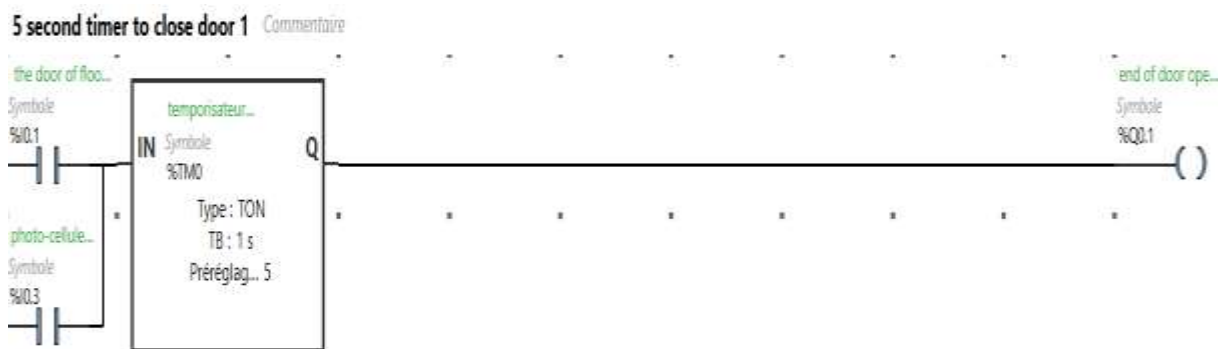
Figure III.12. 5s timer to close door 1 floor
