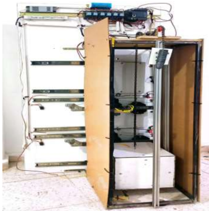
Figure III.2. Back side of the elevator
