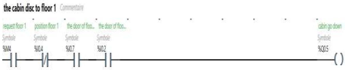
Figure III.6. the cabin amount to floor 1
