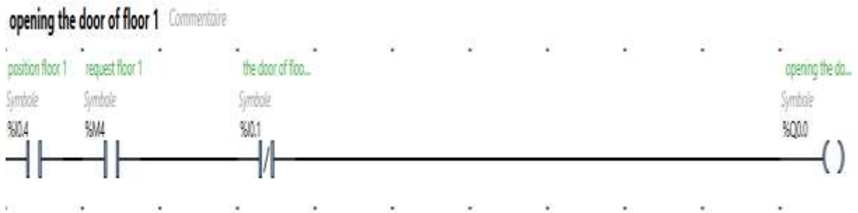
Figure III.10. 1st floor door opening
