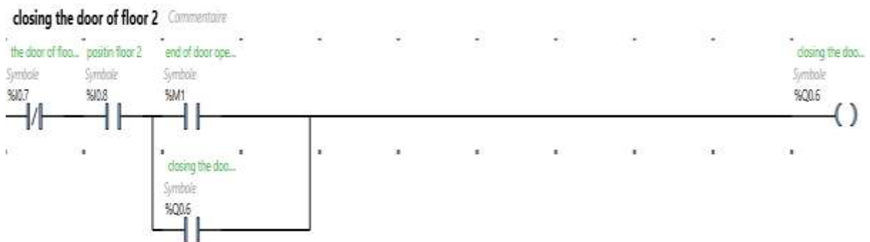
Figure III.9. 2nd floor door closing
