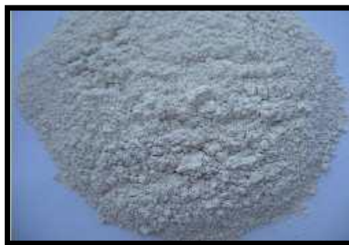
Photo III.6: Cendres volantes de charbon: Point d'origine: Guangdong China (Mainland) [33]
