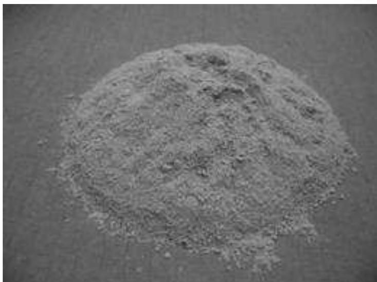
**Figure III.4** Filler calcaire
