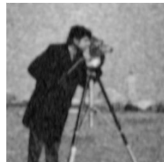
j) filtrage médian de taille (3 \times 3) psnr = 21.12dB snr = 9.55dB ssim = 0.60
