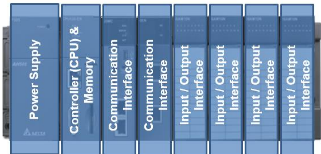
Fig. II. 3 Diagram of Modular Type PLC Architecture
