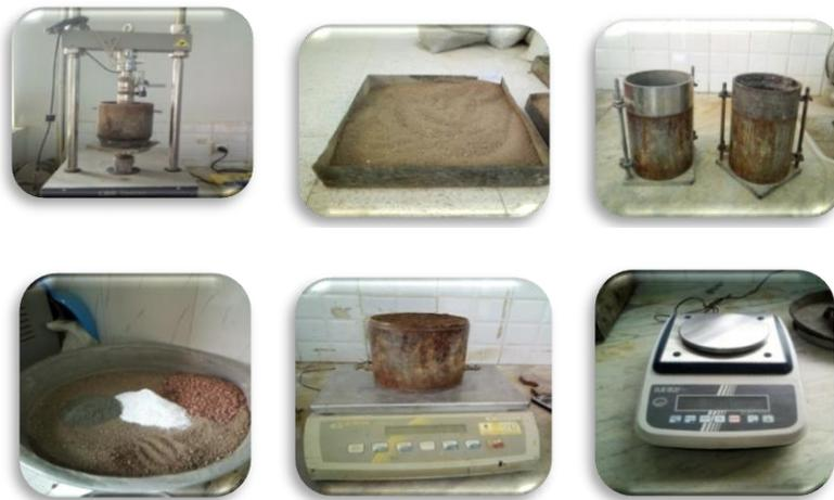
Figure 3.9 : Appareillage – essai Proctor.
