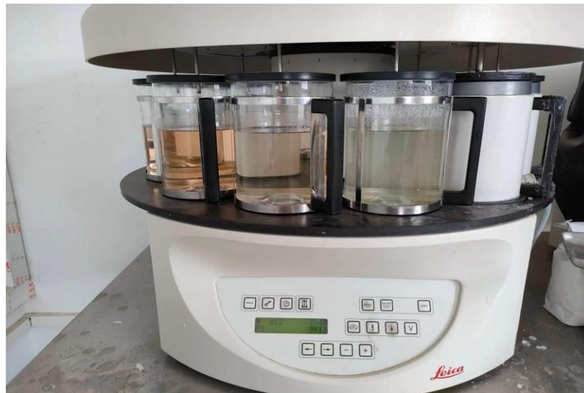
**Figure 2 :** Automate a inclusion (model LEICA TP 1020)
