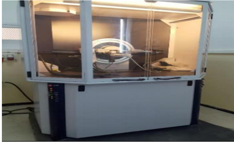
Figure II.5 : Diffractomètre ( Bruker AXS)
