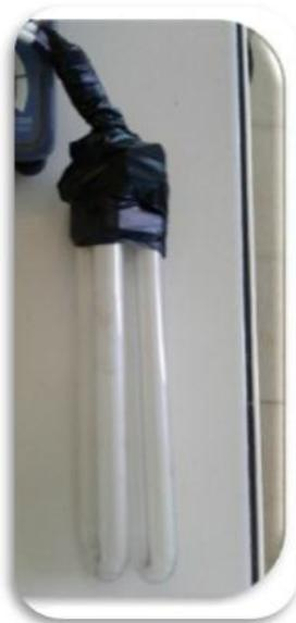
*Figure II.8 :* Lampe UV (12 V, 18 W, 365 nm)
