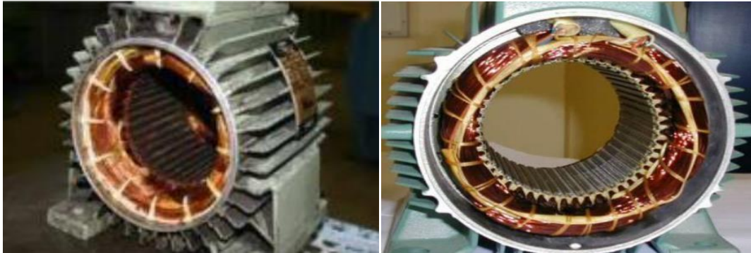
Figure I- 1: Stator de la machine asynchrone .
