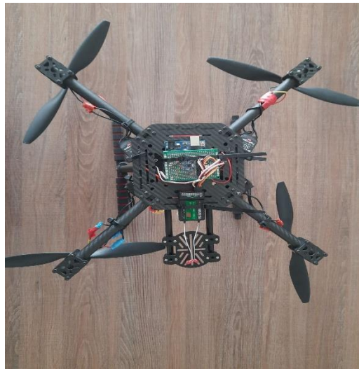
Figure 3-34 The final assembly of flight controller based on Arduino UNO
