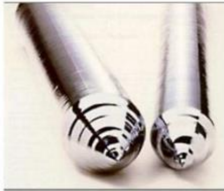
Figure I.8 : lingots de Si monocristallin [14]
