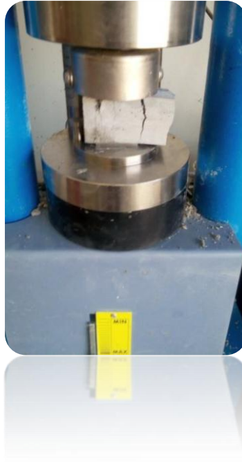
Photo II.5: Essai de compression.
