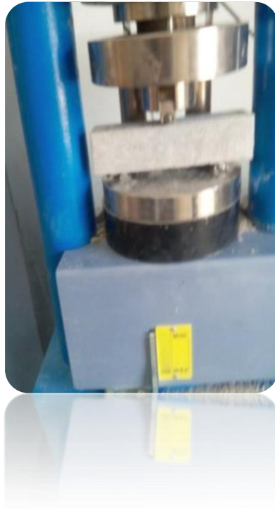
Photo II.4 : Essai de flexion.
