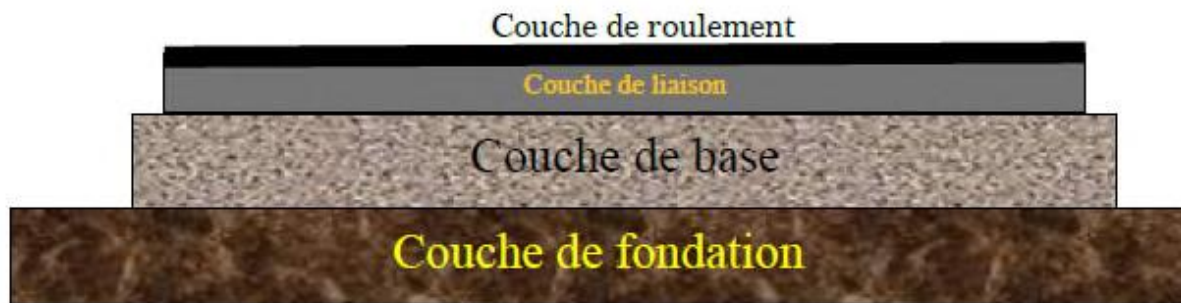
Figure 11 : Chaussée souple. (LCPC, SETRA, Bagnex, 1998).
