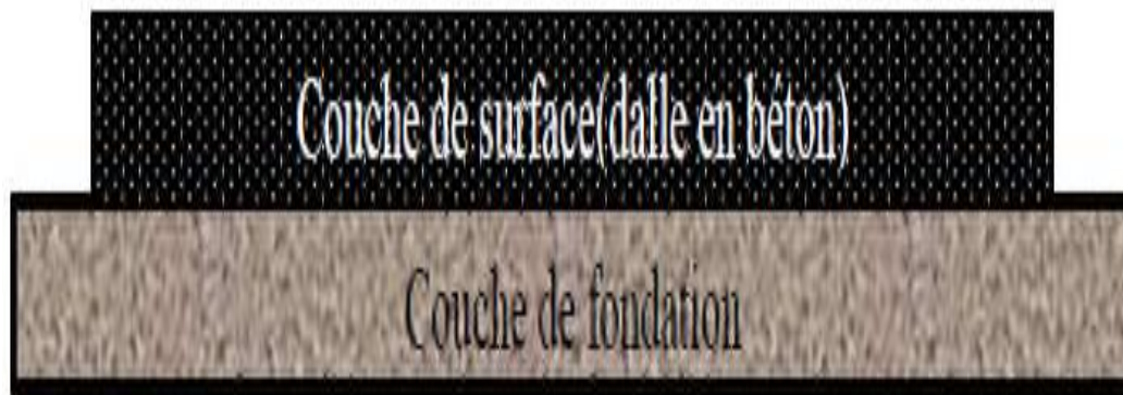
Figure 12 : Chaussée rigide (Barabet, 2012).
