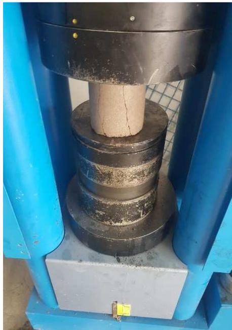
Figure 2.13: Essai de compression.
