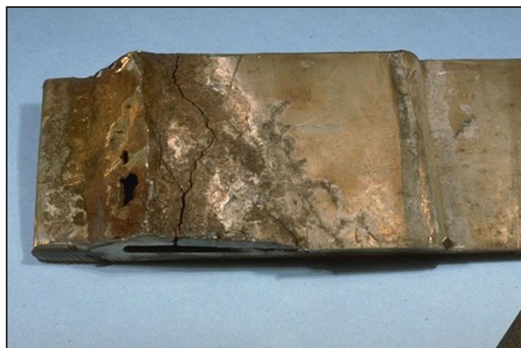
Figure I.4: Corrosion sous contrainte
