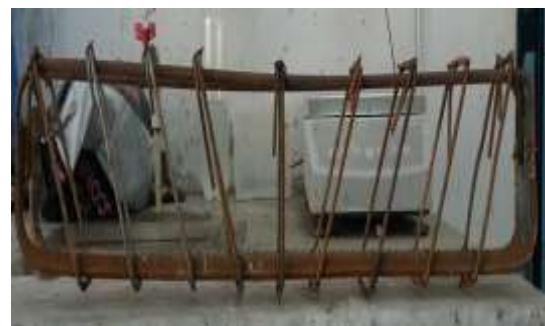
Figure 5.III.2: Ferrailage final de la poutre.
