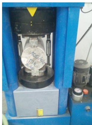
Photo III.14 : Essai de fendage.
