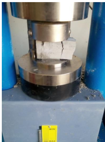
Photo III.9 : Essai de compression.
