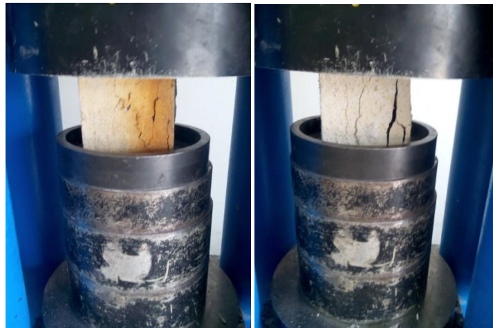
Photo IV.2: Essai de compression.
