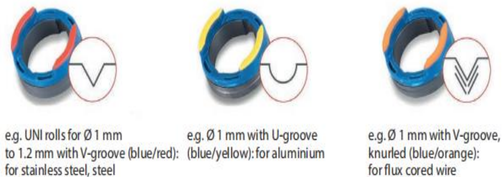
Figure. 2. 9 - Drive rolls with differing groove geometries. [14]
