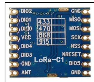
Figure 3.12 : Module Lora SX1276.
