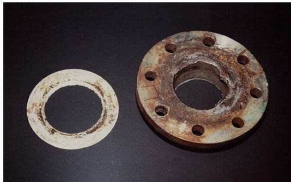
**Figure I.17**: Corrosion cavernueuse.
